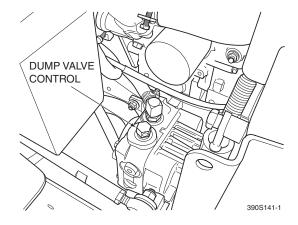
Figure 4-4. Dump Valve Control
